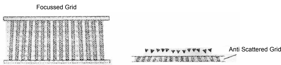
Fig. 2.9.4: Showing focused grid and convergent line
